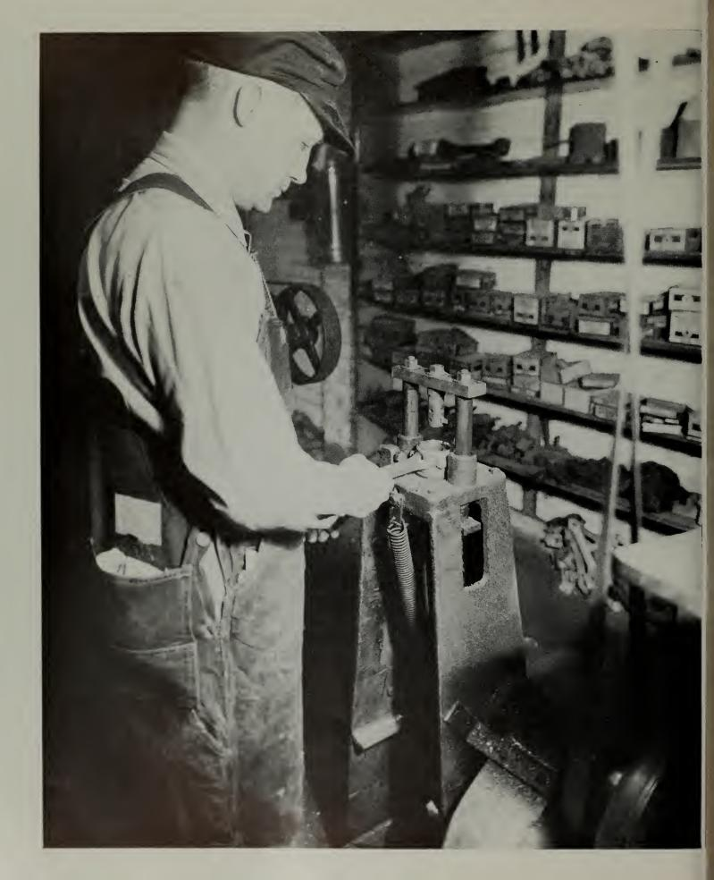
On Model A Ford connecting rods in which the babbitt was cast without the use of separator shims, it is necessary to cut the babbitt through the center of the bearing in order to free the cap from the shank. This operation also leaves an oil groove or relief which facilitates lubrication. This operation is performed by a slotting tool as shown in the above picture.
